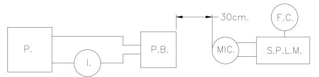
P.: DC Power Supply GPC-3030D or Equivalent S.P.L.M.: Sound Pressure Level Meter IEC651 TYPE2
