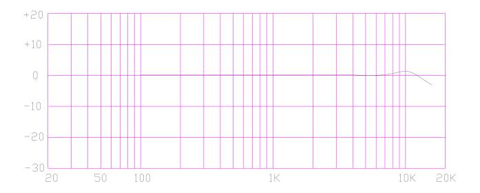
○Frequency: 50~16,000Hz○Max. Operating Voltage: 10V
